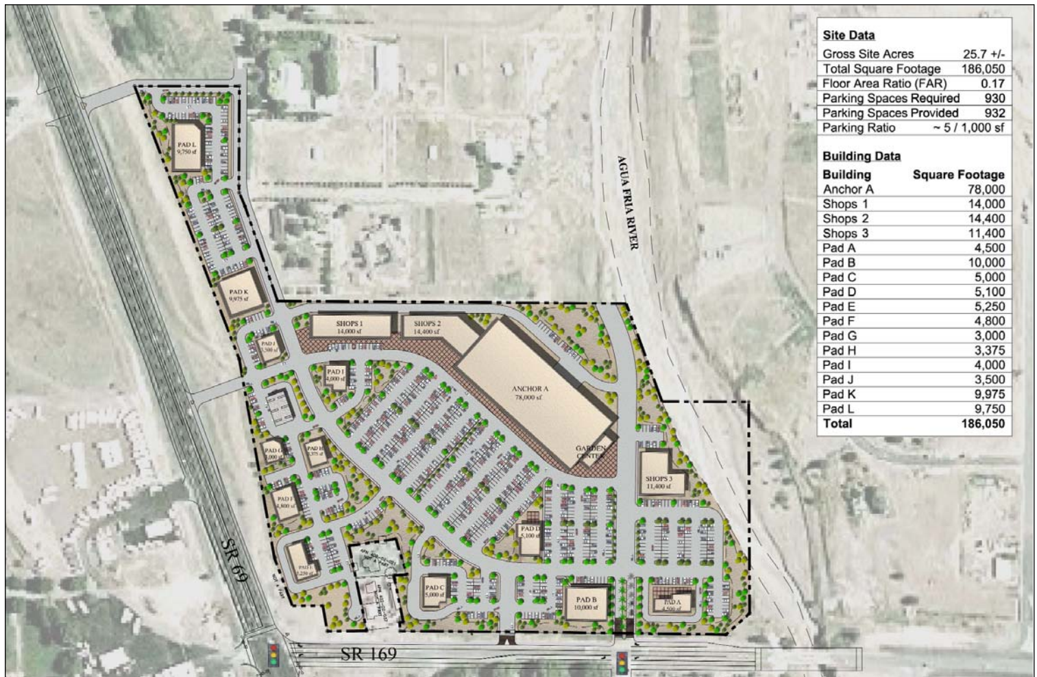
Prescott Valley Crossing Conceptual Site Plan (subject to change) based on current C2-PAD zoning
